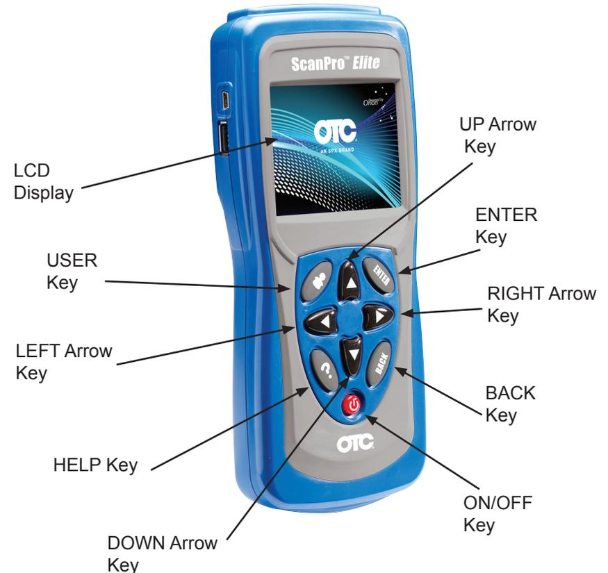
The Quick Start Guide was developed to help you get started using the Scan Tool. If there are any problems following these steps or extra information is required refer to the User's Guide located on the included CD. All Safety Information is contained in the User's Guide. **Read User's Guide completely before operating Scan Tool.**
