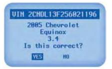
AutoID – Automatically pulls the VIN for most 2000 and newer vehicles and decodes to the vehicle make, model and year so you don't have to
