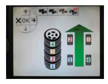
Minimize vehicle drift by letting the balancer tell you the optimal location to put each tire to address conicity issues.
