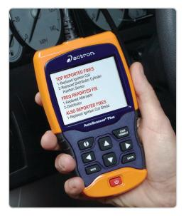
CP9680 indicates on screen which codes have the CodeConnect details. Then it's a simple push of the button to get the CodeConnect information.
