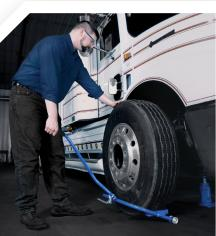
Clever Lever's easy lift and pull action removes the tire. Inside wheels pull off just as easy.
