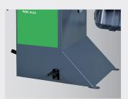
Positioning pedal locks the shaft to eliminate accidental tire roll while applying weights.
