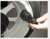
Easy-Fix Auto Locking Weight Positioning arm ensures correct weight placement everytime.
