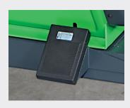
Positioning pedal locks shaft to eliminate tire roll while applying weights
