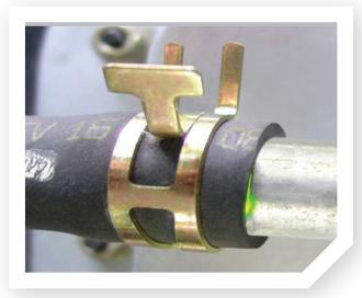
Ultraviolet fluorescent dye fingerprints the exact location of a leak.
