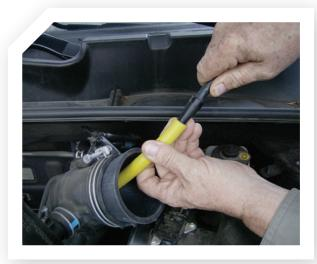
Install appropriate port adapter and insert smoke solution supply hose into adapter.
