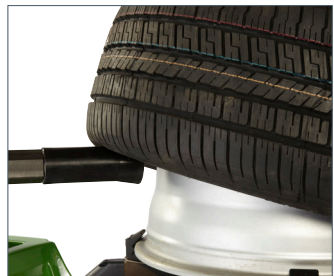
Bead press device and roller provide optimal control while mounting challenging beads
