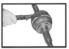
**STEP 4:** Turn tool over to bend band over lock tangs of clamp, as shown in photo above. Do not let band slip back through tool, because this will decrease clamping force.
