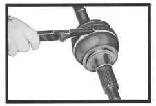
**STEP 4:** Turn tool over to bend band over lock tangs of clamp, as shown in photo above. Do not let band slip back through tool, because this will decrease clamping force.
