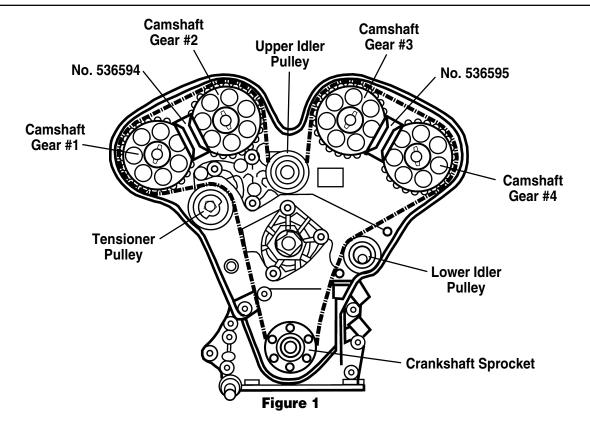
1. With the tensioner pulley loose and No. 536594 and No. 536595 camshaft locking tools in place, install the timing belt following these steps:
