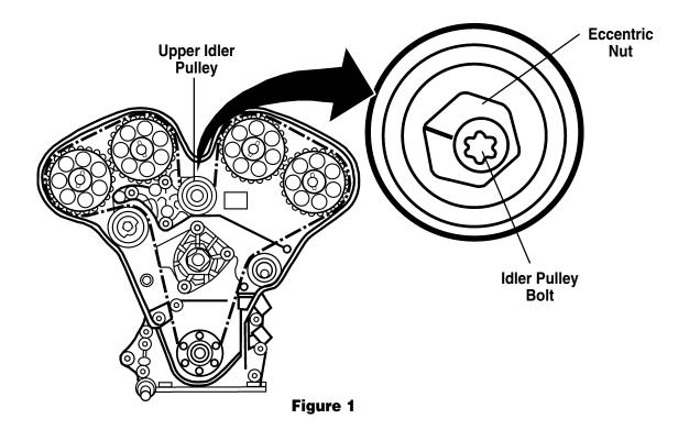
1. Use No. 536612 timing belt tensioner wrench to turn the eccentric nut on the upper idler pulley to set the belt tension. When the belt tension has been set to specification, torque the upper idler pulley bolt to 30 ft. lbs.
