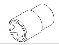
1. Use No. 536613 crankshaft sprocket to rotate the crankshaft as needed when performing the timing procedure.
