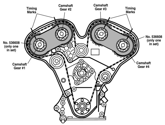
No. 536608 is used to check the camshaft gear alignment—with the timing belt on the engine and tightened to specifications.
