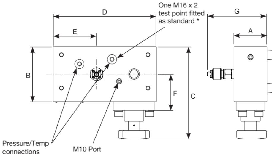
\* Port connected via shuttle valve to ensure maximum pressure is measured regardless of flow direction.
