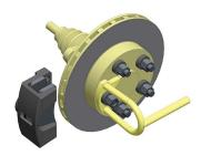
Remove caliper and clean mounting surfaces.
