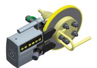
Fit lathe [50 Nm (37 ft-lb)], place drive unit, and machine rotor.
