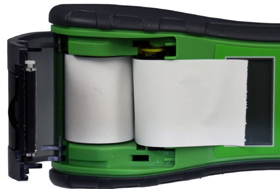
Fig. 4: Paper feeds from underneath the roll
