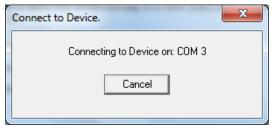
**Note:** If Scanning Suite cannot find the device, you will see a "could not connect to the device" message. If this occurs, try using a different USB port or check Windows Device Manger to ensure the drivers are properly installed and a virtual COM port was created for the Scan Tool.
