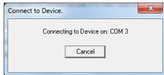
**Note:** If Scanning Suite cannot find the device, you will see a “could not connect to the device” message. If this occurs, try using a different USB port or check Windows Device Manager to ensure the drivers are properly installed and a virtual COM port was created for the Scan Tool.
